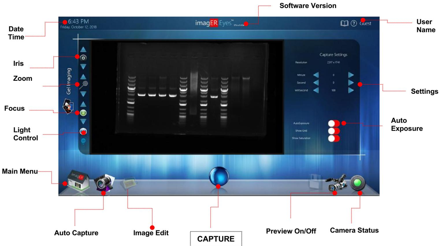
**IRIS:** The iris control adjusts the iris pattern so that it can be clearly seen. Slide the slider up button to open the iris and allow more light to reach the camera sensor and move the slider down button to block the light comes to camera.
