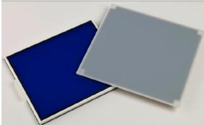
ER Biotech offers a visible light converter that can be placed on top of the UV Transilluminator for imaging Coomassie and silver stained gels.
